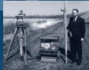
Bob Studebaker with the first rotating laser in the world
